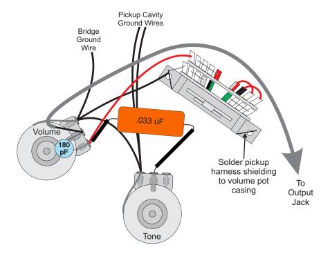
Note Pickup shape is just for reference. All pickups using this diagram shall be oriented in this manner.
